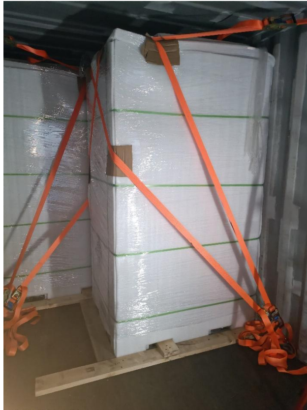
Figure 4-7 Cabinet Loading and Lashing Method Schematic Diagram (3)
