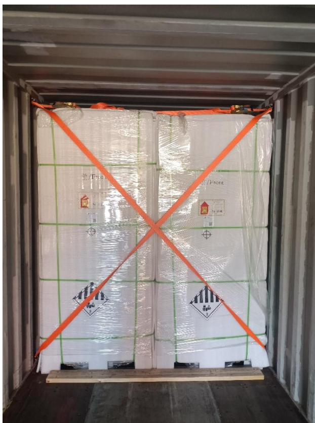
Figure 4-5 Cabinet Loading and Lashing Method Schematic Diagram (1)
