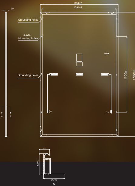
Dimensions of PV Module Unit: mm
